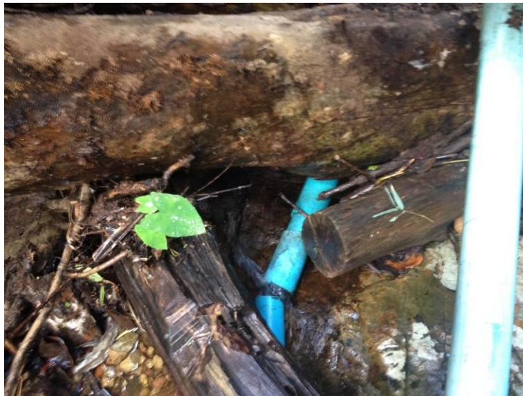
Figure 14: Example of broken pipe section after tree fall
